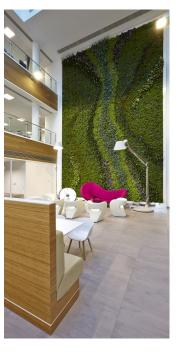
Biotecture's patented hydroponic system allows for each row of modules to drain individually and not onto other modules below. This is unique to Biotecture's green wall system. The advantages are that Biotecture can precisely control moisture levels throughout the wall and ensure that on taller walls, such as Centrica's atrium wall, nutrient levels don't aggregate, which can cause chemical burn to leaves.
